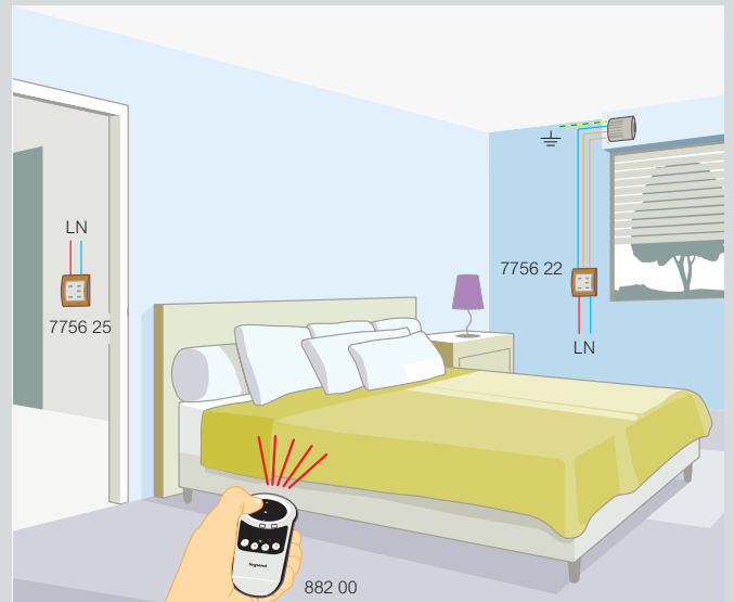
Shutter control in a new building (PLC Solution)
